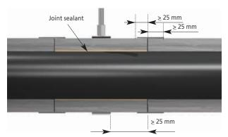
compressive strength of the relevant density and include a safety factor of five. They are designed to support the maximum static compressive loads imposed by horizontal water filled mild steel and copper pipework with hanger supports spaced at the maximum centres shown below. Kooltherm® Insulated Pipe Support Inserts are not designed to accommodate pipe anchor loads and stresses.
