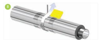
All circumferential seals shall be thoroughly rubbed with a flexible squeegee to ensure a proper vapour tight and lasting adhesion between the tape and the aluminium foil vapour barrier jacket.
