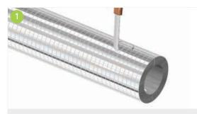
With the longitudinal joint positioned upwards a hole equal to the diameter of the pipe branch shall be made.
