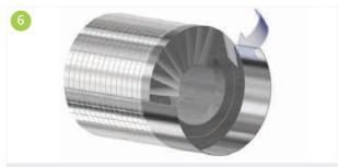
Each tab shall be carefully folded over the end side of the flange box.
