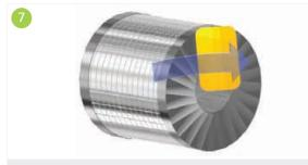
A flexible squeegee shall be used to ensure a proper, vapour tight and lasting adhesion between the tape and the aluminium foil vapour barrier jacket.
