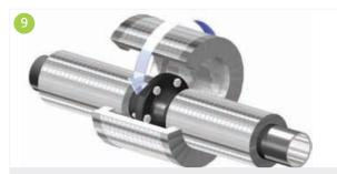
The flange box can be placed on to the pipe. Flanges on horizontal lines are to be insulated with the longitudinal joints facing sideways. Joints should never be facing upwards or downwards.
