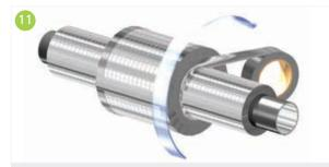
The circumferential joints on both sides shall be individually vapour sealed with an appropriate selfadhesive aluminium foil vapour barrier tape.
