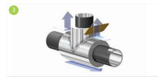
The longitudinal seals shall be thoroughly rubbed with a flexible squeegee to ensure a vapour tight adhesion between the tape and the aluminium foil vapour barrier jacket.
