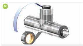
When the adjoining Kooltherm<sup>®</sup> Pipe Insulation sections are fitted and installed, the circumferential joints shall be vapour sealed with appropriate self-adhesive aluminium foil vapour barrier tape.
