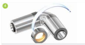
When the adjoining Kooltherm<sup>®</sup> Pipe Insulation sections are fitted and installed, the coinciding circumferential joints shall be vapour sealed with an appropriate selfadhesive aluminium foil vapour barrier tape.
