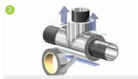
All longitudinal joints shall be vapour sealed with an appropriate self-adhesive aluminium foil vapour barrier tape.
