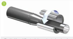
The Kooltherm<sup>®</sup> Pipe Insulation section is placed on the small diameter pipe. Horizontal lines are to be insulated with the longitudinal joints facing sideways to prevent penetration of moisture.
