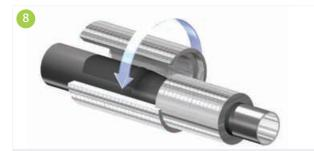
The Kooltherm<sup>®</sup> Pipe Insulation section is permanently fitted over the large diameter pipe with an overlap on the smaller diameter Kooltherm<sup>®</sup> Pipe Insulation section. Care shall be taken that a closed fit is made.
