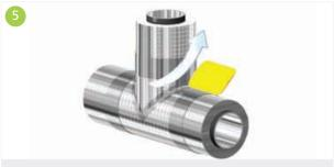
All circumferential seals shall be thoroughly rubbed with a flexible squeegee to ensure a proper, vapour tight and lasting adhesion between the tape and the aluminium foil vapour barrier jacket.
