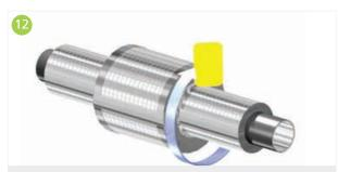
All longitudinal and circumferential seals shall be thoroughly rubbed with a flexible squeegee to ensure a proper, vapour tight and lasting adhesion between the tape and the aluminium foil vapour barrier jacket.
