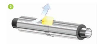
Circumferential seals shall be thoroughly yet gently rubbed with a flexible squeegee to ensure a secure, vapour tight and long-lasting adhesion between the self-adhesive aluminium foil vapour barrier tape and the aluminum foil vapour barrier jacket.
