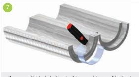
A snap-off blade knife shall be used to modify the inner diameter of the large diameter pipe cover, with a depth equal to the insulation thickness.
