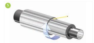
A circumferential marking of the small diameter insulation shall be made on the large diameter front side.
