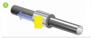
A flexible squeegee is used to ensure a vapour tight and lasting adhesion between the tape and the aluminium foil vapour barrier jacket.
