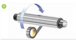
Self-adhesive aluminium foil vapour barrier tape shall be applied centrally at all circumferential butt joints of adjoining Kooltherm<sup>®</sup> Pipe Insulation sections to provide a secure and vapour tight seal.
