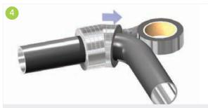
The procedure shall be repeated until the full angle of the elbow is achieved and all longitudinal joints are taped.
