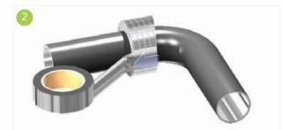
The longitudinal joint of each mitre shall individually be vapour sealed with an appropriate self-adhesive aluminium foil vapour barrier tape.
