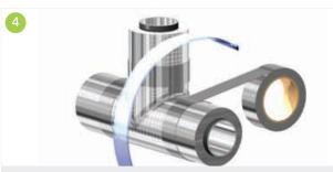
When the adjoining Kooltherm<sup>®</sup> Pipe Insulation sections are fitted and installed, the coinciding circumferential joints shall be vapour sealed with an appropriate selfadhesive vapour barrier tape.
