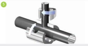
Both parts shall be fitted on the tube with special attention to a closed fit of the coinciding joints.
