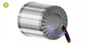
A snap-off blade shall be used to remove the excessive tape.
