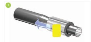
The longitudinal seal shall be thoroughly rubbed with a flexible squeegee to ensure a proper, vapour tight and lasting adhesion between the tape and the aluminium foil vapour barrier jacket.
