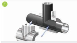
The milled pre-fabricated Kooltherm<sup>®</sup> tee, made in two halves shall be positioned onto the pipe. Care shall be taken that no gaps arise and a closed fit is ensured.
