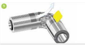
The connecting circumferential seal shall be thoroughly rubbed with a flexible squeegee to ensure a proper, vapour tight and lasting adhesion between the tape and the aluminium foil vapour barrier jacket.
