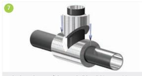
The branch part of the tee shall be slid into position with special attention to a properly closed fit of the joints.
