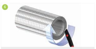
A snap-off blade knife shall be used to modify the inner diameter of the large diameter pipe cover, with a depth equal to the insulation thickness.
