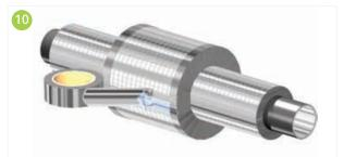
The longitudinal joints shall be individually vapour sealed with an appropriate self-adhesive aluminium foil vapour barrier tape.
