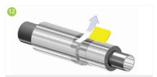
All longitudinal and circumferential seals shall be thoroughly rubbed with a flexible squeegee to ensure a proper, vapour tight and lasting adhesion between the tape and the aluminium foil vapour barrier jacket.
