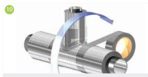
WWhen the adjoining Kooltherm<sup>®</sup> Pipe Insulation sections are fitted and installed, the circumferential joints shall be vapour sealed with appropriate self-adhesive aluminium foil vapour barrier tape.
