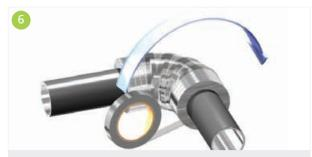
All circumferential joints shall be vapour sealed with an appropriate self-adhesive aluminium foil vapour barrier tape. Enough pressure shall be used on the mitred parts to properly close the circumferential joints.
