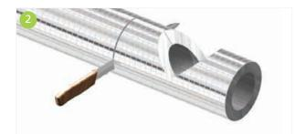
The length of the main part shall extend at least 50 mm on each side of the branch to facilitate a vapour sealed joint. A clean vertical cut shall be made.
