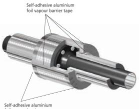
Self-adhesive aluminium foil vapour barrier tape, folded over the end sides in strips cut to size.
