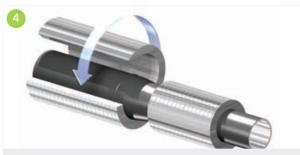
The Kooltherm<sup>®</sup> Pipe Insulation section is temporarily fitted over the large diameter pipe and slid against the small diameter Kooltherm<sup>®</sup> Pipe Insulation section.
