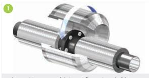
The Kooltherm<sup>®</sup> pre-fabricated flange box shall be placed on the pipe. Flanges on horizontal lines are to be insulated with the longitudinal joints sideways to prevent penetration of moisture.
