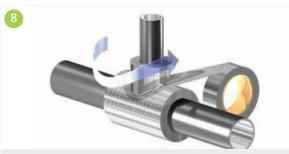
The coinciding joint shall be vapour sealed with an appropriate self-adhesive vapour barrier tape. Enough pressure shall be used to ensure full contact between the insulation parts.
