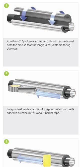
To ensure maximum adhesion and without crushing the insulation, gently pull the self-adhesive aluminium foil vapour barrier tape tight to seal all joints, and with a flexible plastic spatula / felt squeegee gently exert the necessary amount of pressure.
