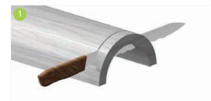
Two filling rings shall be cut with a minimum length equal to the insulation thickness of the adjoining insulated pipe.
