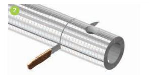
The length of the main insulation part shall extend at least 50 mm on each side of the insulated branch to facilitate a vapour sealed joint. A clean vertical cut shall be made.
