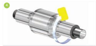
All longitudinal and circumferential seals shall be thoroughly rubbed with a flexible squeegee to ensure a proper, vapour tight and lasting adhesion between the tape and the aluminium foil vapour barrier jacket.
