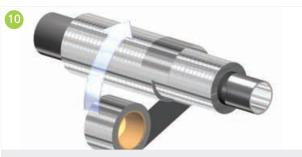
An appropriate self-adhesive vapour barrier tape shall be applied over the coinciding circumferential joint. Width of the tape shall be selected to facilitate a minimum 25 mm cover on both sides of the circumferential joint.
