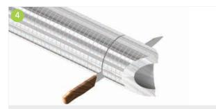
The length of the branch shall extend at least 50 mm to facilitate a vapour sealed joint. A clean vertical cut shall be made.
