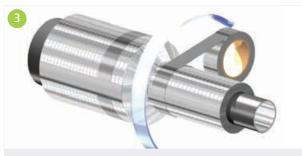
The circumferential joints on both sides shall be individually vapour sealed with an appropriate selfadhesive aluminium foil vapour barrier tape. Kooltherm<sup>®</sup> milled fittings have 50 mm extended ends to facilitate a proper fit to the adjoining pipe covers.
