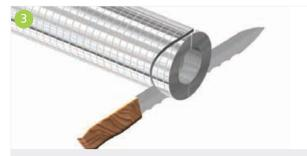
A curved cut is made identical to the outer surface of the insulation on the main pipe.
