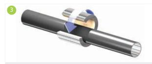
The Kooltherm<sup>®</sup> Insulated Pipe Support Inserts are placed on the pipe. Support inserts on horizontal lines are to be insulated with the longitudinal joints facing sideways.
