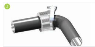
When positioning the next tapered insulation element, care shall be taken that a proper fit is made and no gaps arise in the joints.
