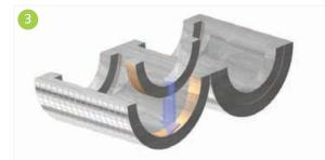
The filler rings shall be glued into the oversized ring with appropriate contact glue.
