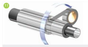
The bridging self-adhesive vapour barrier tape shall be secured with an additional seal onto the small diameter Kooltherm<sup>®</sup> Pipe Insulation section.
