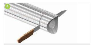
The length of the branch insulation part shall extend at least 50 mm to facilitate a vapour sealed joint. A clean vertical cut shall be made.
