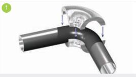
The milled Kooltherm<sup>®</sup> pre-fabricated elbow shall be placed into position. Care shall be taken that no gaps arise and a close fit is made.
