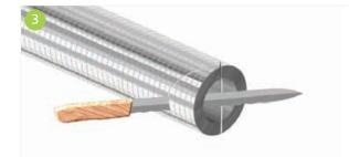
The branch of the tee shall be made by two clean vertical 45° angled cuts.
