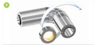
When the adjoining Kooltherm® Pipe Insulation sections are fitted and installed, the circumferential joints shall be vapour sealed with an appropriate self-adhesive aluminium foil vapour barrier tape.
