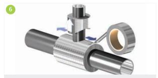
The longitudinal joints of both parts shall individually be vapour sealed with an appropriate self-adhesive aluminium foil vapour barrier tape.
