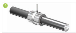
When the clamp is installed, care must be taken that the aluminium foil vapour barrier jacket of the Kooltherm<sup>®</sup> Insulated Pipe Support Inserts is not damaged in any way.
