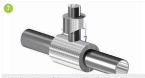
The branch part of the tee shall be slid into position with special attention to a closed fit of the joints.
