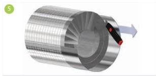
A snap-off blade knife shall be used to divide the selfadhesive aluminium foil vapour barrier tape into small tabs.
