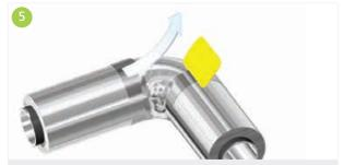
The circumferential seals shall be thoroughly rubbed with a flexible squeegee to ensure a proper, vapour tight and lasting adhesion between the tape and the aluminium foil vapour barrier jacket.
