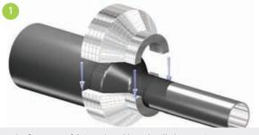
The factory pre-fabricated Kooltherm<sup>®</sup> milled eccentric or concentric reducer, made in two halves, shall be positioned onto the pipe. Care shall be taken that no gaps arise and a close fit is made.
