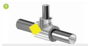
All seals shall be thoroughly rubbed with a flexible squeegee to ensure a proper, vapour tight and lasting adhesion between the tape and the aluminium foil vapour barrier jacket.
