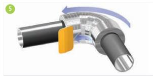
All seals shall be thoroughly rubbed with a flexible squeegee to ensure a proper, vapour tight and lasting adhesion between the tape and the aluminium foil vapour barrier jacket.
