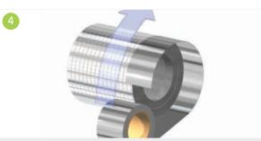
Self-adhesive vapour barrier tape shall be applied at both ends of the flange. The width of the tape shall be selected to facilitate full sealing of the ends.
