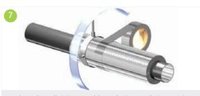
When the adjoining Kooltherm® Pipe Insulation sections are in place, the coinciding circumferential joints shall be vapour sealed with an appropriate self-adhesive aluminium foil vapour barrier tape.
