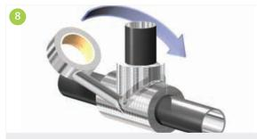
The joints of both parts shall be vapour sealed with an appropriate self-adhesive aluminium foil vapour barrier tape.
