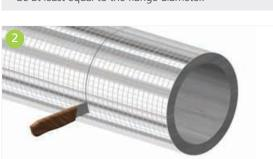
The oversized Kooltherm® Pipe Insulation section shall be cut to length. A clean vertical cut shall be made.
