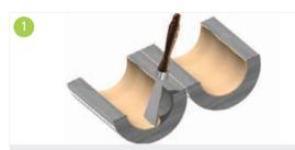
For cold applications, the inner surface of the Kooltherm<sup>®</sup> Insulated Pipe Support Inserts shall be fully coated with an appropriate joint sealant.
